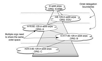
Figure 2: The  $m\langle masklength \rangle$  technique and RFC 2317 allow us to split authority between octets.
